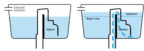
If in the unlikely event that your filling valve fails to close, all Delchem siphons feature an internal overflow which will be able to cope with upto 35l/min of excess water.
