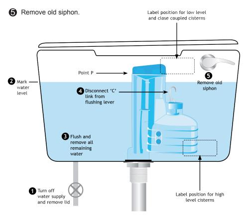
**Note:** When using internal overflow in the siphon ensure that point 'P' is below all apertures in the walls of the cistern
